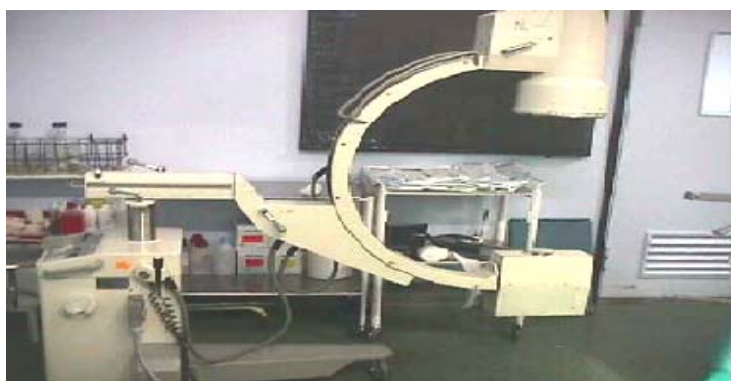
Figure1. Demonstrating A Mobile C-Arm Fluoroscopic Unit- Ziehm Exposcop / Cb7-D
